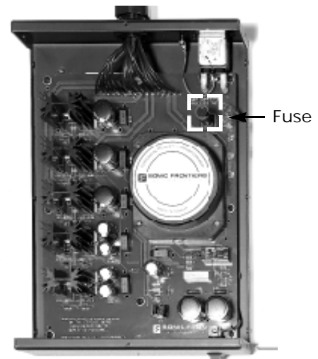
Figure 9 - The Fuse in the Processor 3 is located in the right rear corner of the power supply chassis.
